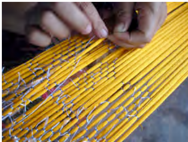
Figure 2: Detail of tie-dyeing threads before being woven into mudmee fabric
